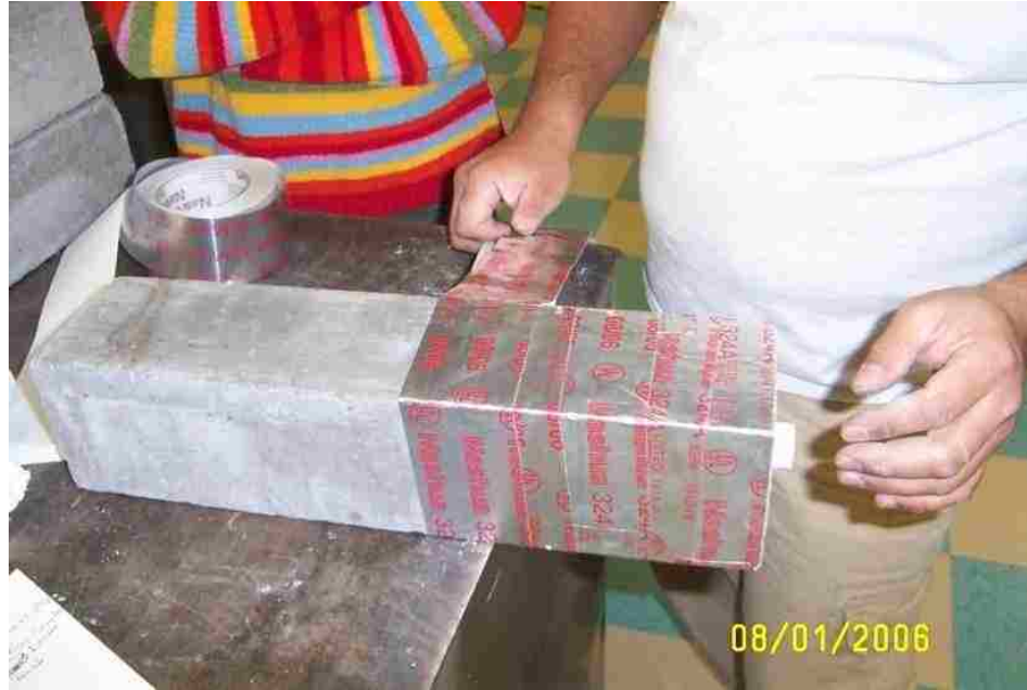
Figure 3.7. Sealing of sealed specimens with aluminium tape
